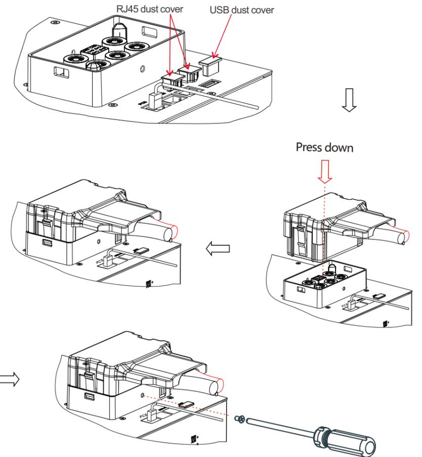
Note: 1) Please install the communication line first, then plug the unused RJ45 port and USB port with a dust cover, and finally install the power line.
