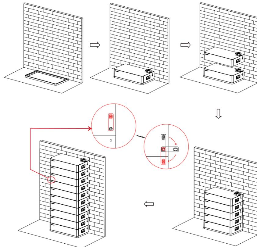
Note: When stacking, make sure that all batteries are aligned and lock the safety bolt.
