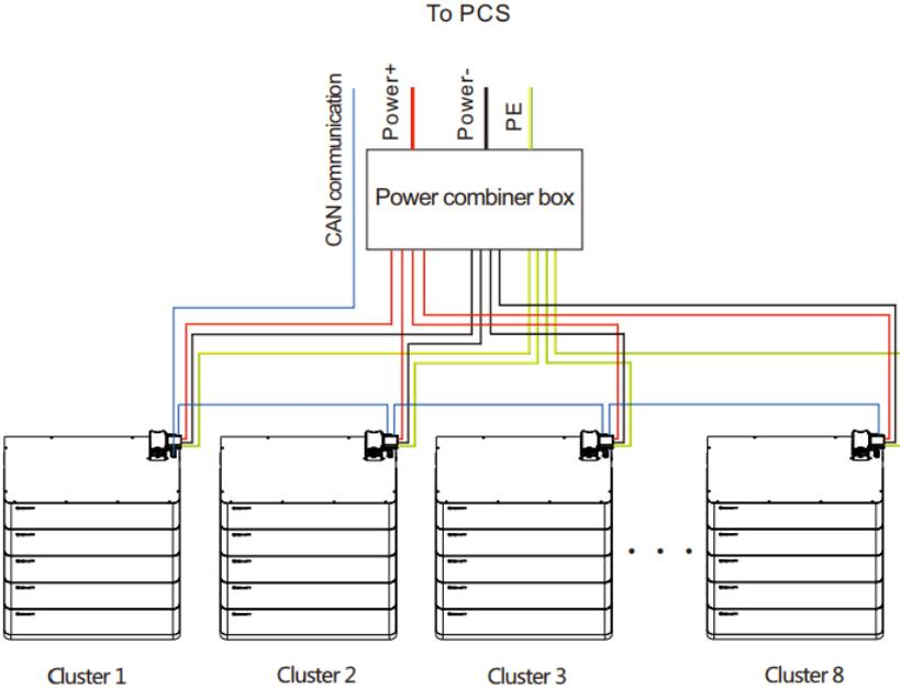
Figure 14: Block diagram of multi-cluster system
