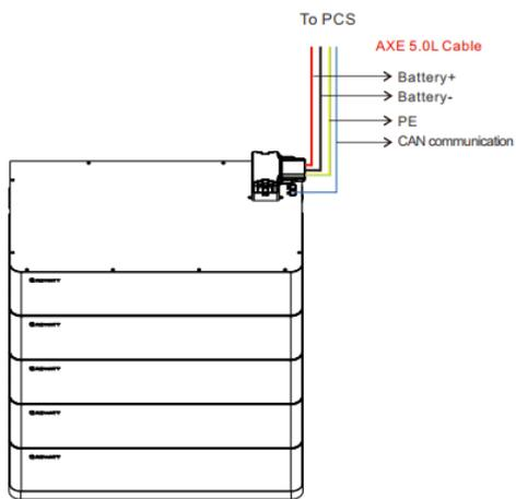
Figure 11: Block diagram of a single cluster system
