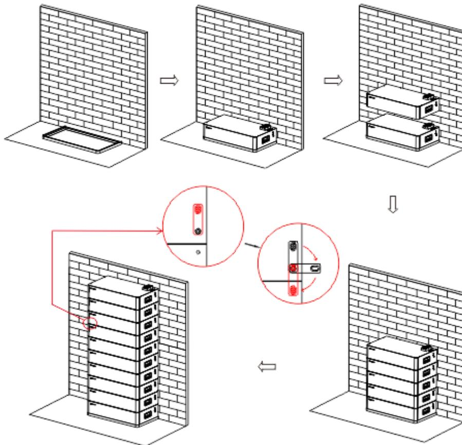
Figure 10:Multiple AXE 5.0L with base installation process
