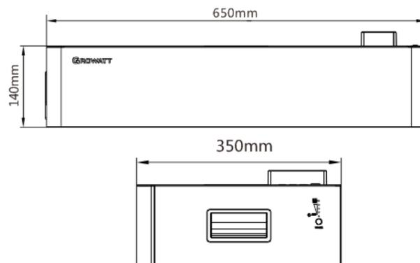
Figure 1: Battery size diagram
