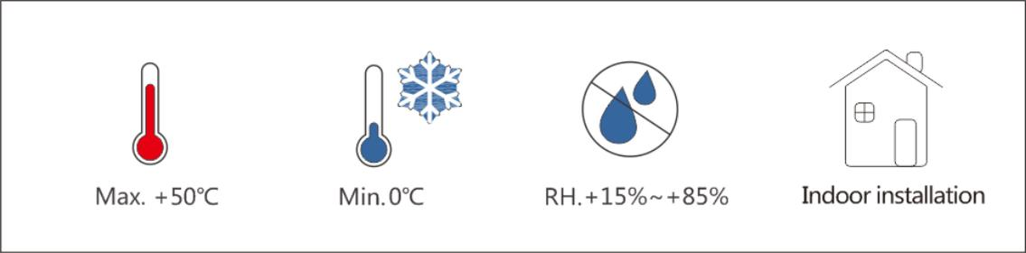
Fig 6: Installation environment requirements
