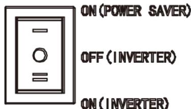
Once the unit has been properly installed and the batteries are connected well, simply press On/Off switch (located on the button of the case) to turn on the unit.
