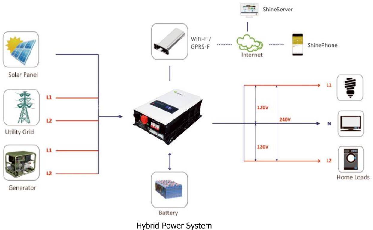
This is a multifunctional split-phase output off grid solar inverter, integrated with a MPPT solar charge controller, a low frequency pure sine wave inverter and a UPS function module in one machine, which is perfect for off grid backup power and self-consumption applications.
