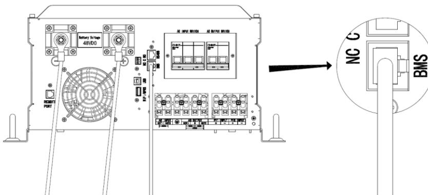
4. The other end of RJ45 insert to battery comm port.
