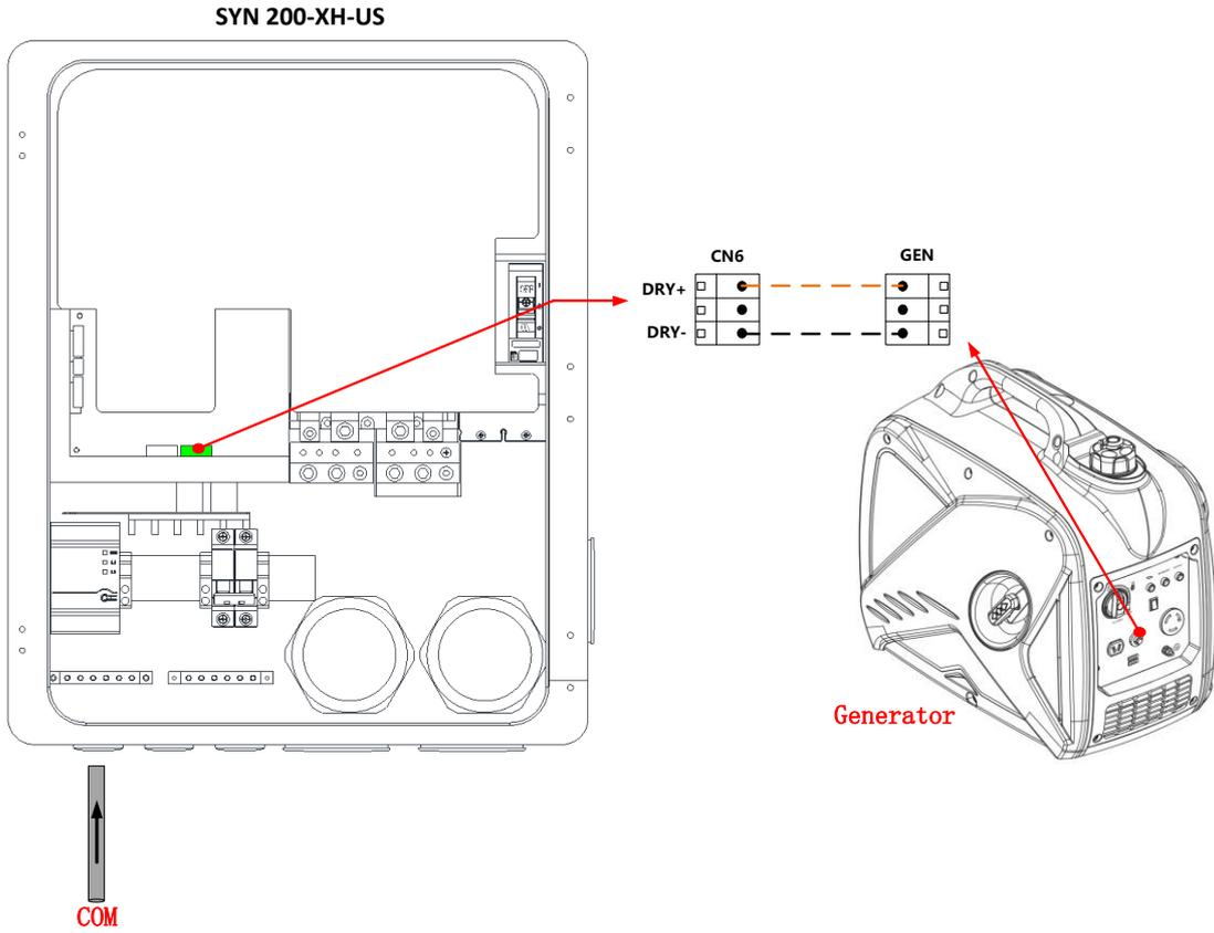
Communication connection between Backup Interface and Generator
