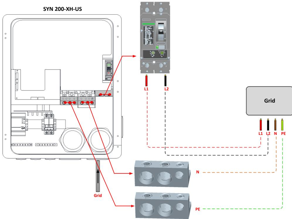
Connection to the Grid (Contains AC breaker)
