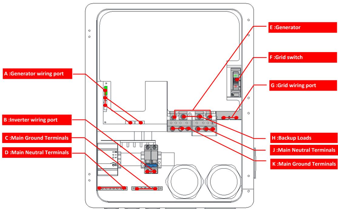
Internal wiring diagram
