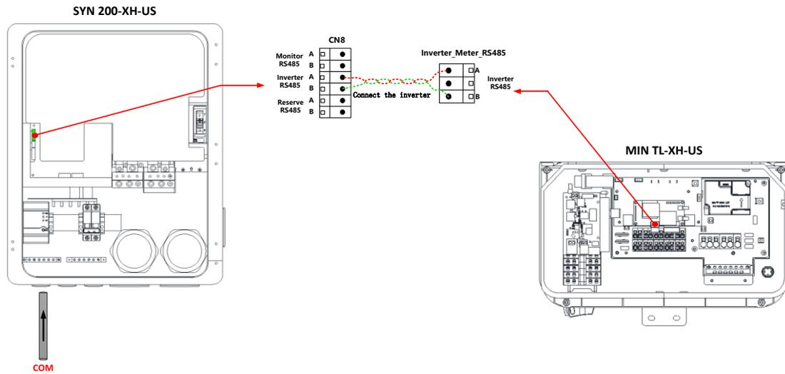
Communication connection between Backup Interface and Inverter
